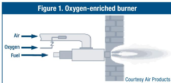
Figure 1. Oxygen-enriched burner
